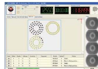
Support various PCB board type, includes, LED boards up to 1200 mm long (or option to 1800mm), flexible PCB , or circular PCB
