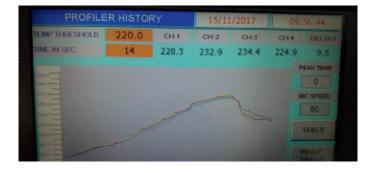
Optional 4 channel profiler allows full screen display of 4 thermocouple inputs on-line and also displays  $\Delta T$ .
