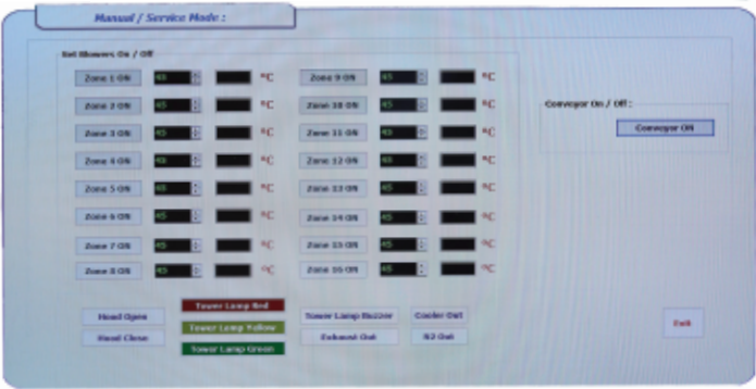
Manual or Service Mode of operation, which is Password protected, available for independently checking almost all operations - blowers, hood, tower lamp, cooler, chain lubrication etc allowing easy maintenance & troubleshooting of faults at any section.
