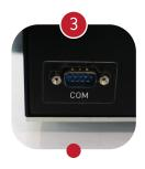
External connection for communication with ultrasonic welding machines, barcode reader or PC programming using Excel™ files
