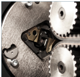
High precise rotary incision unit based on industry leading Schleuniger technology
