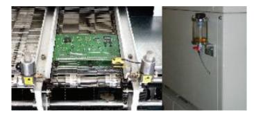
Automatic chain lubricating system, controlled by computer and can be programmed. Supply of oil from glass jar at the back of machine.
