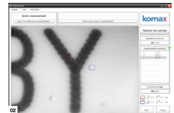
01 UV laser marked wire 02 Contrast measured by the EasyContrast system provided by Komax
