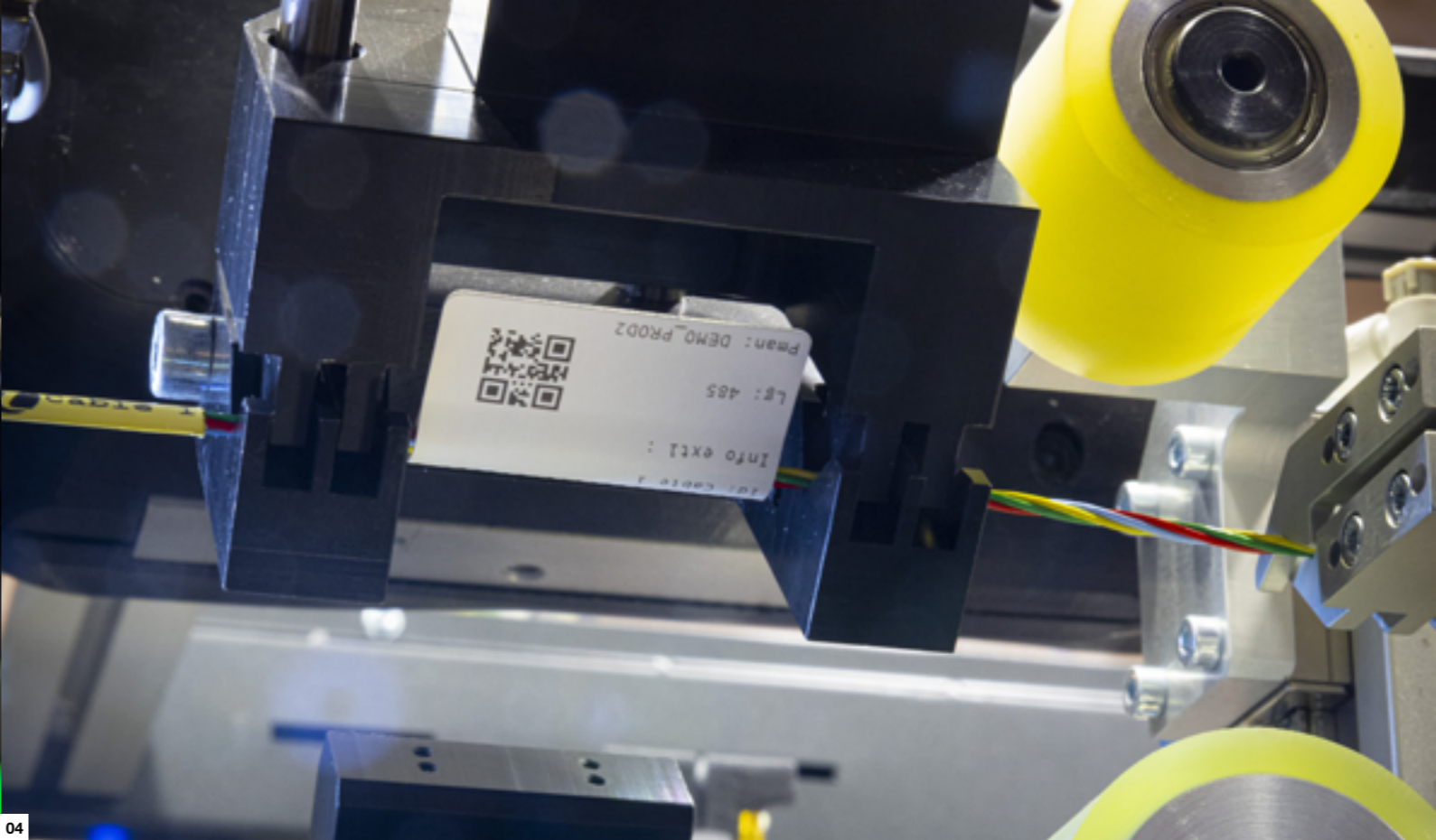
04 The WEL module automatically labels wire extremities with customizable content.
