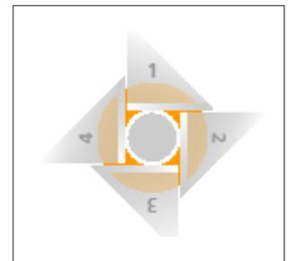
Because of the 4 blades (large contact surface), even thin and strongly adhering insulations can be removed.
