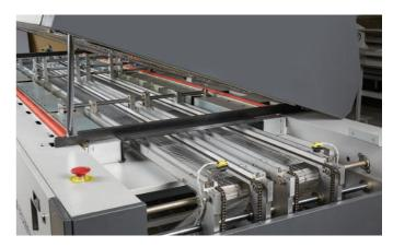
Dual Conveyor Setup - Unique to EMS Technologies Reflow ovens, the dual conveyor setup allows for two simultaneous boards to be passed at the same time thus increasing throughput leading to increased productivity. The dual conveyor setup can be configured to two different sizes of PCB with independant width control as well as independant speed control offering versatile application as per application demand.
