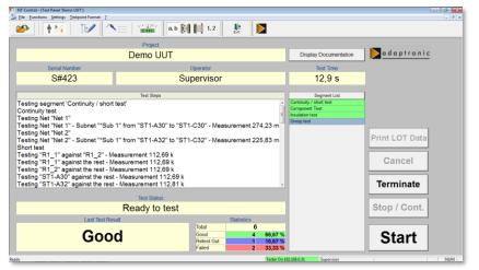
Operation within test mode via buttons which can be activated with mouse-click or with the touch function of a touch screen.
